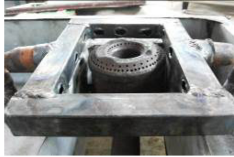
Fig 17. Grill with flue gas passage
