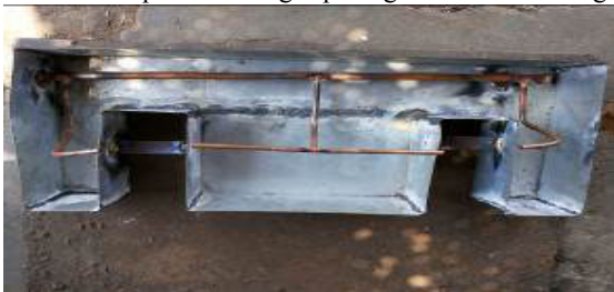
Fig 16. Fabricated water chamber with flue gas passage (Stove I)
